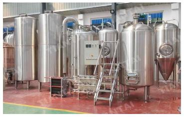
In the Brew kettle the wort is boiled with the addition of hops.
