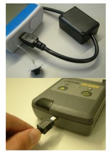
Press the \$\mathbf{\Gamma}\$ button at your humimeter until you reach the menu (see image on the right). Choose "Print Logs" and confirm by pressing \$\mathbf{-}\text{l}\$.
