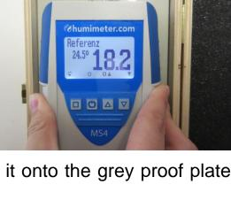
Press the third button until the black bar has reached the first digit of your serial number. After a waiting time of a few seconds the device accepts the entered digit. Now the other 3 digits have to be entered. When the 4-digit number has been entered correctly (see picture), press the + button to confirm.
