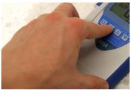
Select the right calibration curve using the buttons ▲ or ▼. The name of the calibration curve is shown at the top of the display. To enter the list of calibration curves, press one of the arrow keys for 3 seconds.
