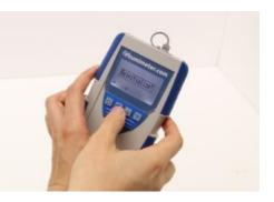
Hold the humimeter MS4 in one hand up in the air and make sure that nothing stands behind the sensor plate. Then confirm the query "Calibrate?" by pressing the second button ( $\checkmark$ ) with one finger.
