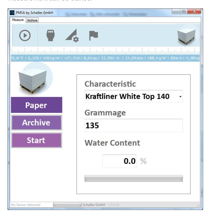
First of all choose the corresponding characteristic curve for the paper to measure. Clicking the arrow in the field Characteristic, a list with all available calibration curves opens. Select the desired curve by clicking on it.
