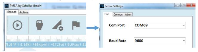
After choosing the correct COM port, the connection between hardware and software can be tested by clicking the button "Test". If the test was successful, this is shown by a popup window and by the LED status bar shining in blue. Then click the "Save" button.
