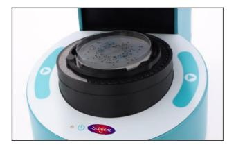
After pushing the button, the diffusing sphere (2) will descend to cover the Petri dish, the lighting and image acquisition procedures will be performed, and finally, the diffusing sphere will return to its upper resting position. Then the process results will be displayed on the screen.
