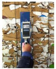
4.) Measurements can be taking at different positions of the paper bale as outlined in Step 3. The measurements can be saved in the store menu by pressing the button on the handle bar. The saving of data can is complete when the number in front of the symbol increases.
