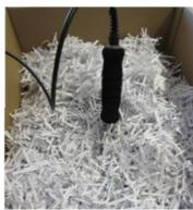
Plug the sensor into the material to measure and let it adjust for approx. 15 minutes. Turn-On the humimeter RP6 device and select the desired calibration curve. The display immediately shows the measurement.
