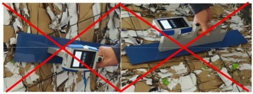
□ Connected USB cable during measuring
