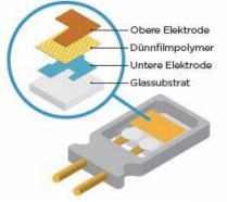
Dirt on the sensor doesn't influence the accuracy, but increases the reaction time. Devices using capacitive humidity sensors are: <u>AW1, AW2, AW3, RH2, RH5, RH6, RH1, Marathon Dataloggers</u>, <u>Scigiene Wireless Systems</u>
