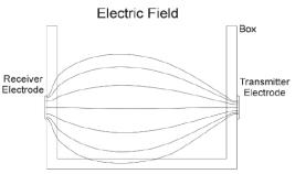
sensor, building an electric high-frequency field (dielectric) in the material to measure.
