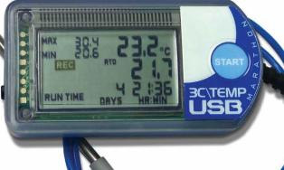
Temperature Range Internal Sensor: -29°C to +72°C External probe: -40°C to +300°C
