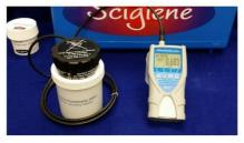
Step 4: Turn on to Log Readings To Stability; typically < 5 minutes
