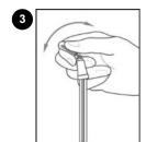
3. Activate Device. Bend bulb, breaking Snap-Valve.
