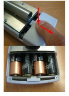
If the battery symbol appears in the measuring window resp. if a critical charge of battery is shown in the status, the batteries have to be changed IMMEDIATELY. If you do not use your humimeter device for a longer period, remove the batteries. For eventual resulting damages we cannot provide any warranty.
