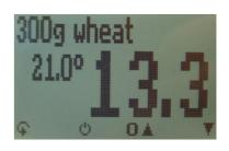
9. If the measuring value is blinking, the valid measuring range has been exceeded (limits see list on page 5). In this case the accuracy is decreasing.
