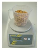
7. Fill up the measuring device with the sample material. The filling needs to be done slowly and constantly to ensure reproducible results.
