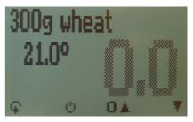
6. Fill up the cup with the sample material (+/- 1.0g). The filling quantity needed is shown on the upper left corner of the display of the device.
