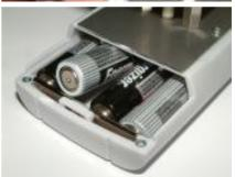
If the battery symbol appears in the measuring window resp. if a critical charge of battery is shown in the status, the batteries have to be changed IMMEDIATELY.
