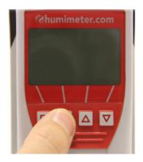
3. Switch on the device by pressing the power button (  $\bigcirc$  ) for 3 seconds.
