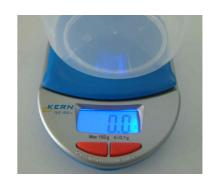
2. Make sure that the measuring chamber is completely empty. It is important that no material is left in the measuring chamber when you turn on the device.
