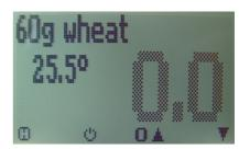
6. Fill up the cup with the sample material (+/- 0.5g). The filling quantity needed is shown on the upper left corner on the display of the device.
