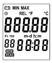
$\overline{-+}$ : The Battery is not sufficient for proper operation.
