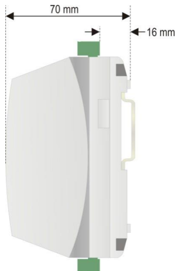
Figure 5 – Dimensions of FieldLogger side without HMI module
