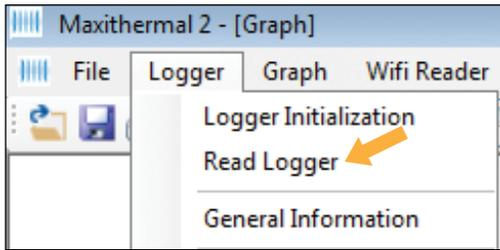
Begin by starting the MaxiThermal software, connect the USB cable, then connect the Marathon data logger.
