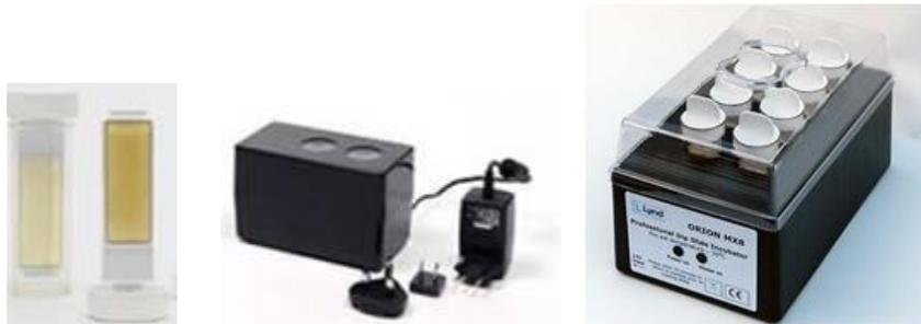
**Method:** For environmental surfaces, the slides are flexible on both sides to tap on the surface. Unscrew the cap, tap the surface gently and put it back. Incubate in upright position using the incubator at required temperature and duration.
