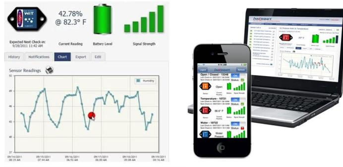
And because its cloud based one or more supervisors can view the readings and receive alerts live from anywhere! A typical system will use our [Temperature sensors](#) for each CCP to be monitored and one or more [Receivers](#) at key points to relay the signals from the sensors to Cloud based software. From here data is streamed to the cloud for local or remote viewing using the software. You can receive alerts on emails (for free) and/or through e-mail or text alerts.
