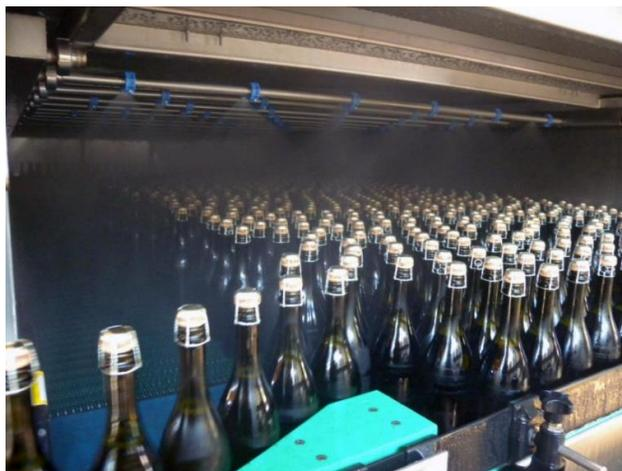
Ideally the process involves measuring internal bottle/can temperature relative to the external temperature of the spray and many processes involve recording internal product temperatures as well. ([SterilDisk](#) and [PasteurDisk](#)) dataloggers inside a dummy can/bottle or an outside probe ([SterilCyl](#), [PasteurCyl](#)) inserted through special fittings to record internal temperatures are ideal here.
